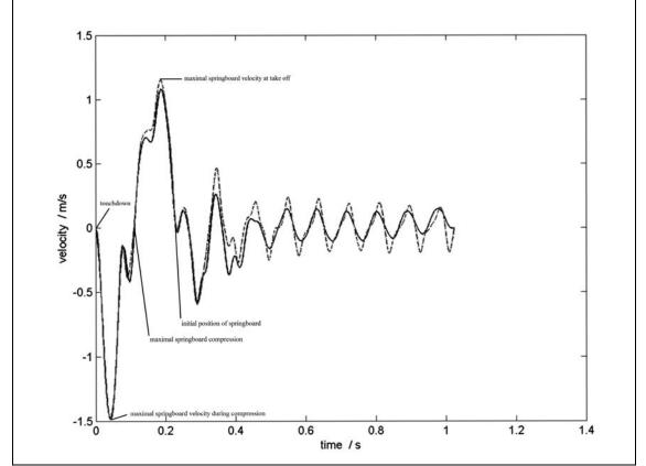
*Figure 3.* A typical velocity vs. time curve obtained with laser (black line) and accelerometer (grey doted line).
