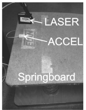
*Figure 2.* Measurement setup - an optical laser sensor placed directly above the acceleration sensor and pointing a laser beam onto the acceleration sensor.
