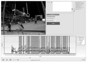
*Figure* 2. Example of automatic determination of the hold time (marked parts of the force-time curve) and synchronized video.
