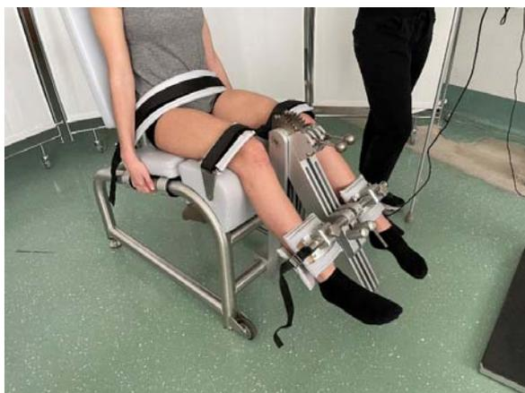
Figure 1. Participant in the isometric knee dynamometer.
