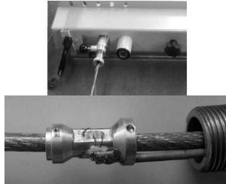
*Figure 1.* Position of the force sensors.
