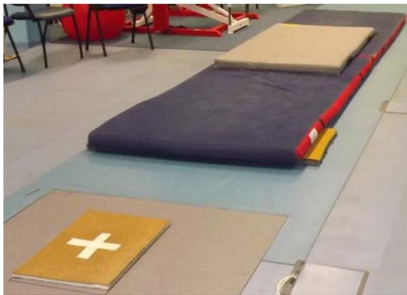
Figure 1. Force plate with a thin floor mat, and mat for back handspring and landing.
