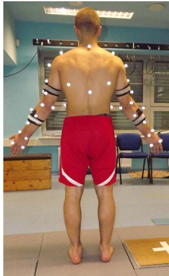
Figure 3. Marker placement on gymnast body.
