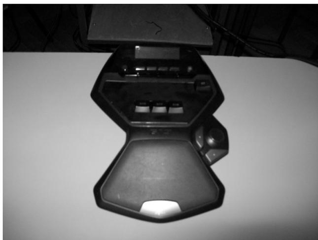
Figure 1. A special keyboard for the entry of deductions (4 keys only, for deductions of 0,1; 0,3; 0,5 and 1 points, respectively).
