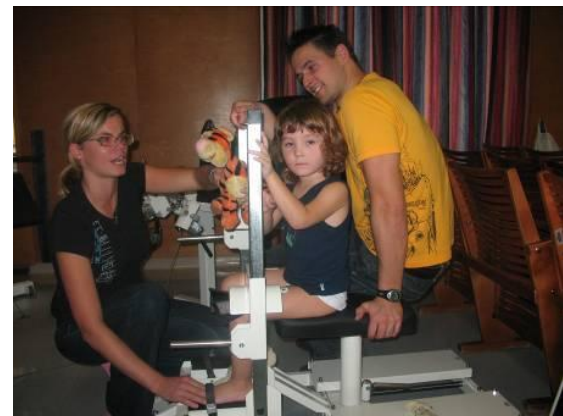
Figure 3: Maximum voluntary torque measurement in knee extension (left) and ankle plantar flexion (right)
