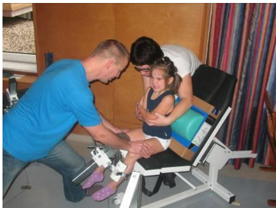
Figure 3: Maximum voluntary torque measurement in knee extension (left) and ankle plantar flexion (right)
