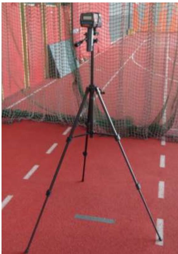
Slika 8. Radar Stalker ATS Professional Sports, katerega smo uporabili na meritvah.
